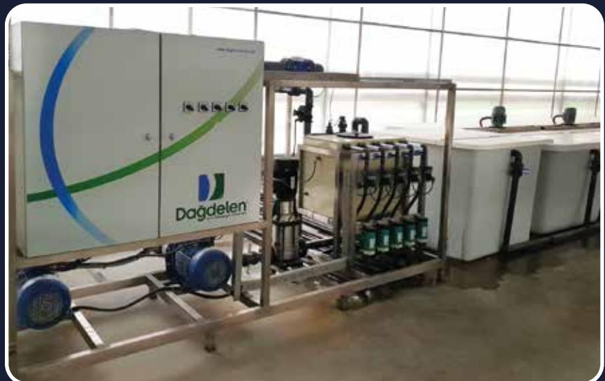
When it reaches the limits determined by using the EC-PH values taken from the sensors fixed on it, it interrupts the flow to the mixing tank and ensures the flow of the fertilizer back to the fertilizer tank through recycling. In this system, instant and more precise dosing is performed. A more homogeneous plant nutrient solution is obtained by premixing water and fertilizer with the mix tank system.
