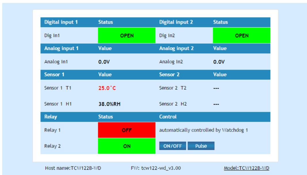
The “Monitoring” page provides information about the state of the relays and digital inputs, values of analog voltages (applied on analog inputs), temperature and humidity.
