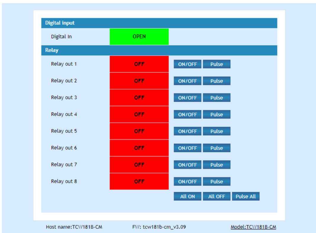
The “Monitoring” page provides information about the state of the relays and digital input.
