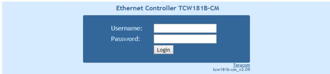
After opening the “Login” page, authorization data must be entered (by default username=admin, password=admin). It is recommended to change the username and password to prevent unauthorized access to the controller. Up to fifteen 1-byte UTF-8 symbols can be used.
