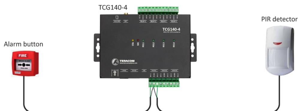
The maximum cable length for a digital input should be up to 30 meters.
