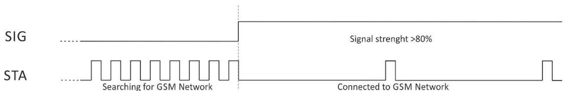
STA flashes twice for 200mS in a period of 2s – there are GSM and 4G/3G/2G connections.
