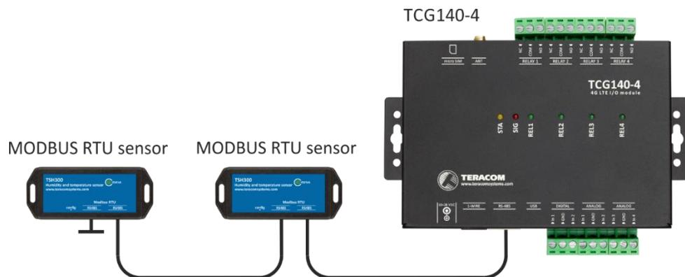
Interconnections are realized by UTP/FTP cables with RJ-45 connectors. The popular Ethernet wiring standard ANSI/TIA/EIA T568B is used.
