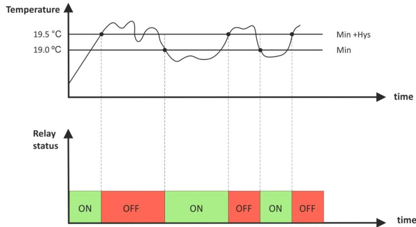
The “Max” value is set far enough from the wanted temperature to avoid trigger/alert conditions around it.
