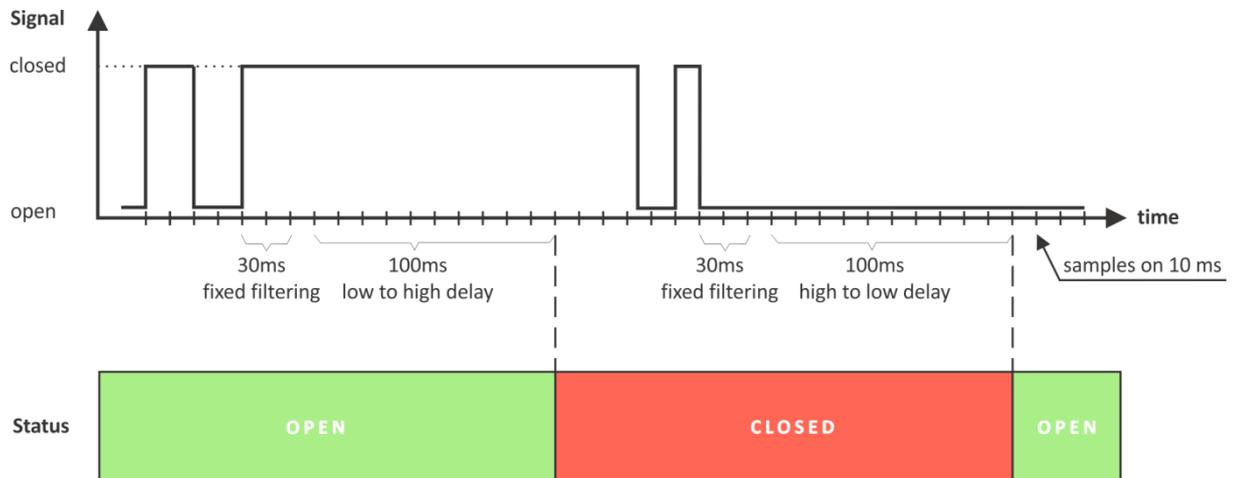
On the picture above low-to-high and high-to-low delays are set to 0.1 seconds.
