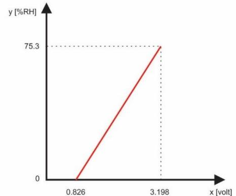
The sensor provides raw voltage values as output, but what we actually need is the corresponding relative humidity values. To achieve this, we use a multiplier and an offset. These two parameters allow us to calculate the relative humidity for any given voltage within the sensor's working range.
