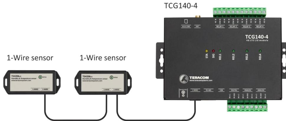
It is strongly recommended to use only UTP/FTP cables and keep the total cable length up to 30m. Although functionality has been achieved in the longer distance, we cannot guarantee error-free operation over mentioned wiring length. We recommend reading Maxim’s 1-Wire tips at <https://www.teracomsystems.com/wp-content/uploads/1-wire/guidelines-for-reliable-long-line-1-wire-networks.pdf>.
