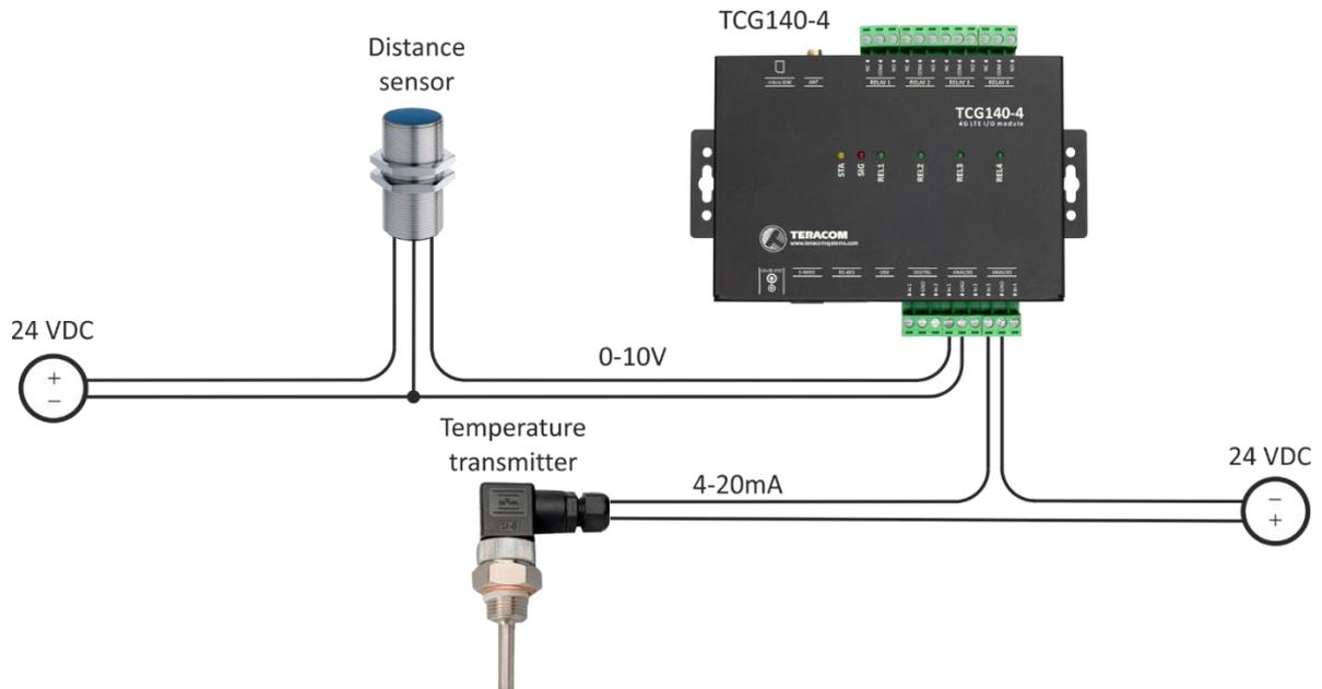
The maximum cable length for an analog input should be up to 30 meters.
