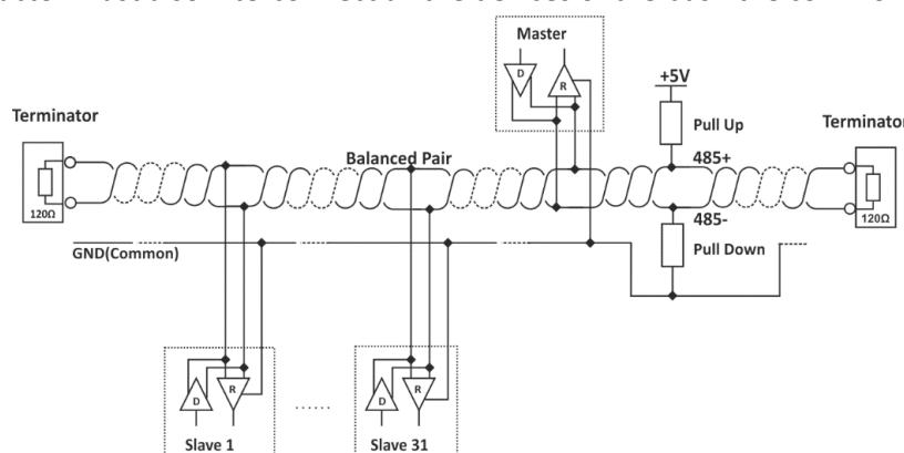
It is highly advisable to use a daisy-chain (linear) topology along with UTP/FTP cables when connecting multiple sensors. To ensure the interface functions correctly, terminators (120-ohm resistors) must be installed at both ends of the bus. The device comes equipped with a built-in 120-ohm resistor, and for bus termination, the terminals "485-" and "Term" should be shortened.
