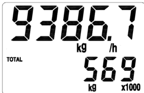
Picture 4.6 Displaying the left digits, a “x1000” mark is displayed
