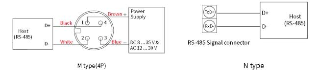
When output of ordering code is RS-485(without analog), RS-485 diagram of default setting is M type.
