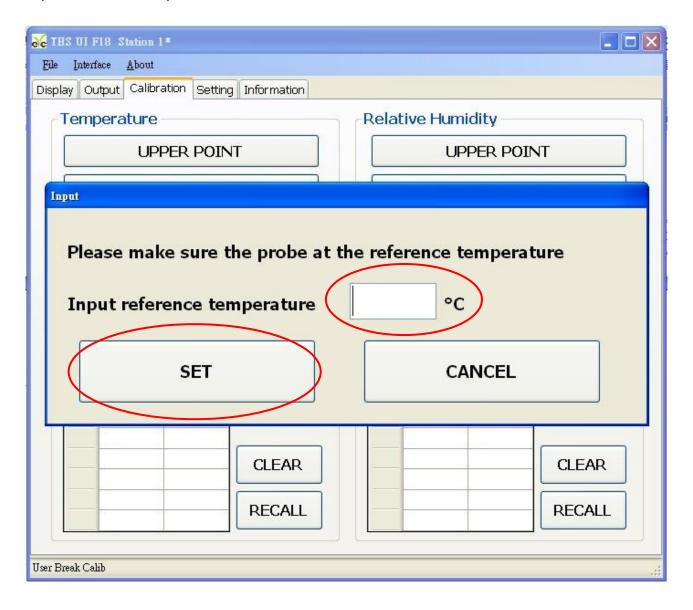
6. That calibrating signal point temperature is done.
