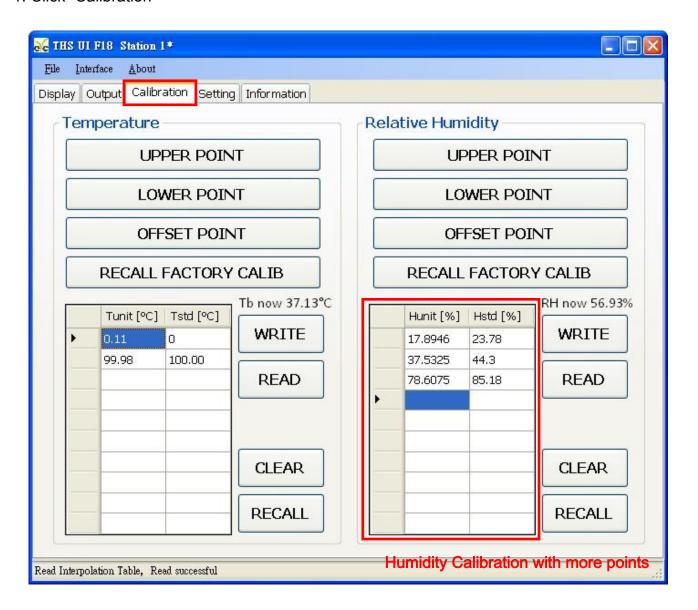
Statement: The existing value is record of more points of calibrating which was executed by factory when operators log in Calibration page at the first time.
