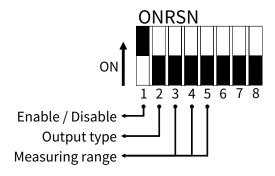
For FTS140 products, the setting status of DIP switch will be read by software while power on, and this reading action will not happen later on. Thus in order to read the DIP switch status again by software, the user must to reboot again if re-setting the DIP switch. The function of DIP Switch\_2 to 5 only be effective
